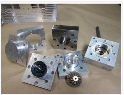
Modular blocks for processing and sampling of gases and liquids, and more specifically to devices allowing rapid construction of fluid reactors, distillers, extractors, homogenizers, filtration/separation devices, and process models.
