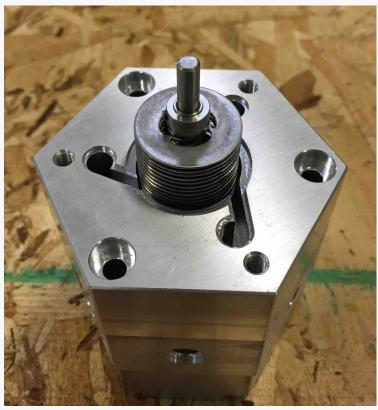
Revolutionizing Fluid Dynamics: This Modular Block features stacked discs designed for noncavitation fluid pumping, drawing inspiration from Tesla's groundbreaking original invention to efficiently pump or expand fluids without loss of performance or integrity.
